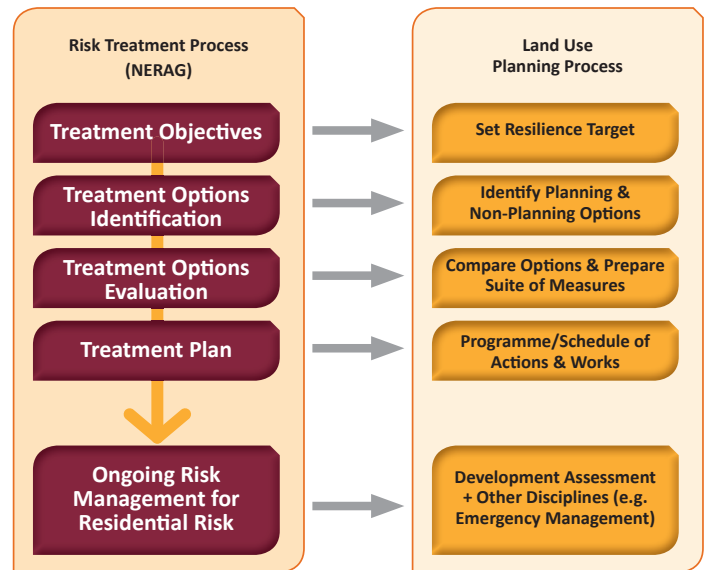
Fig 28: Integrating the land use planning process with the NERAG risk treatment process
