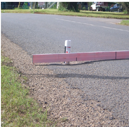
Use of straight edge, taken close up and angled level with the damage
