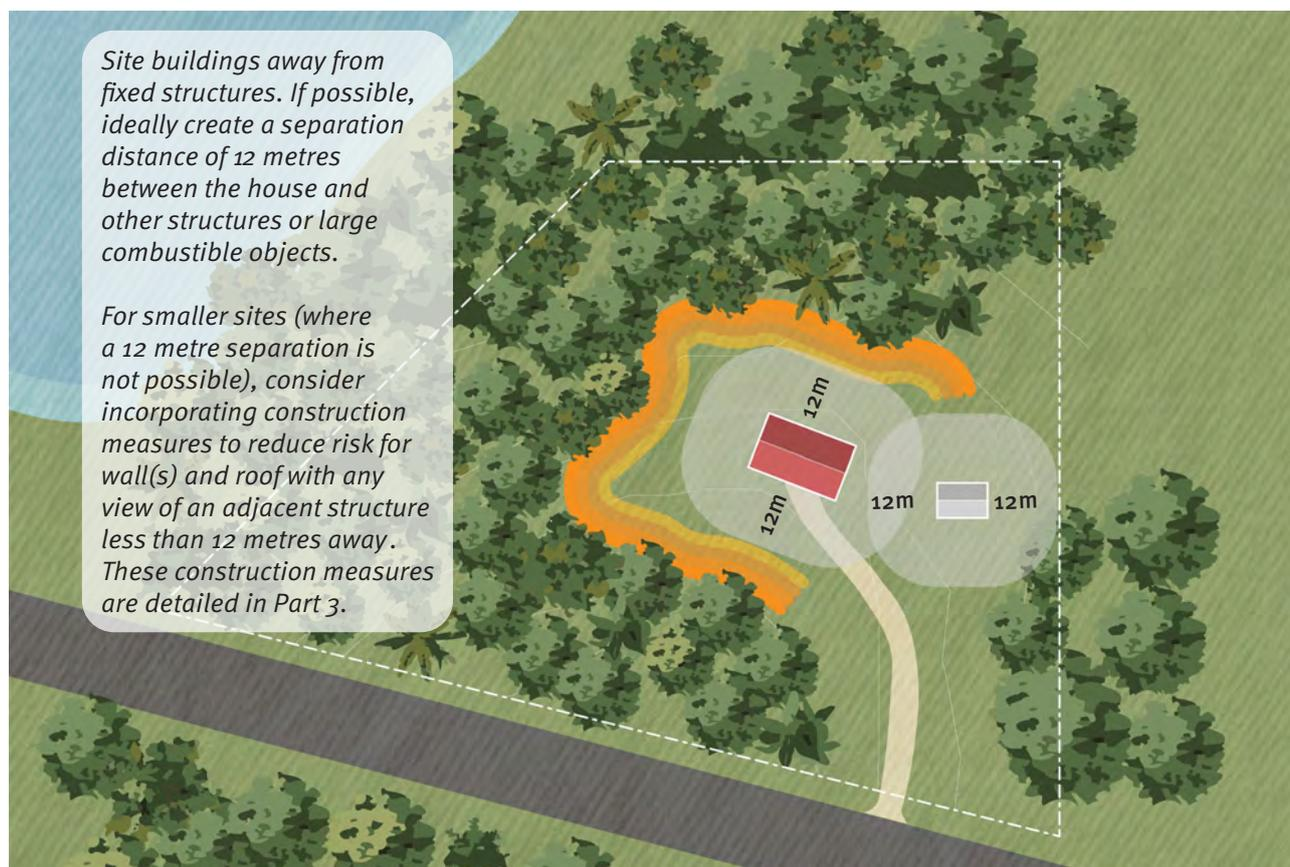
Figure 9 Siting for existing structures<sup>19</sup>
