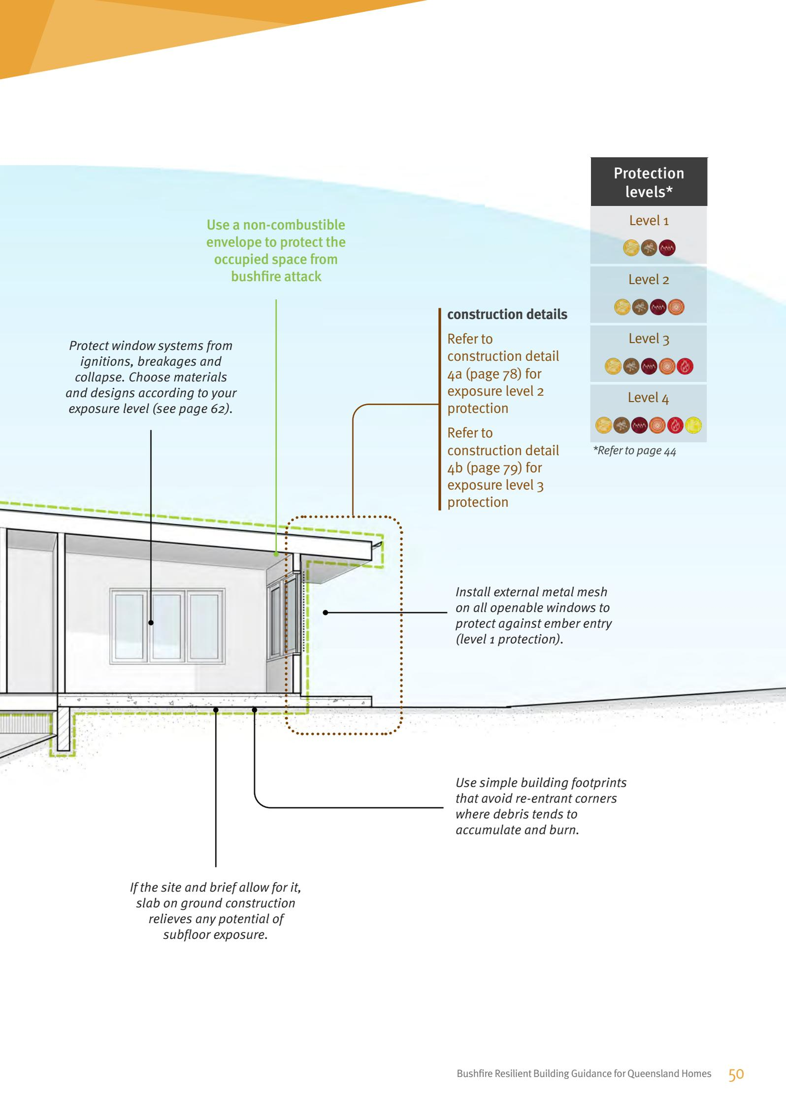
Use a non-combustible envelope to protect the occupied space from bushfire attack
