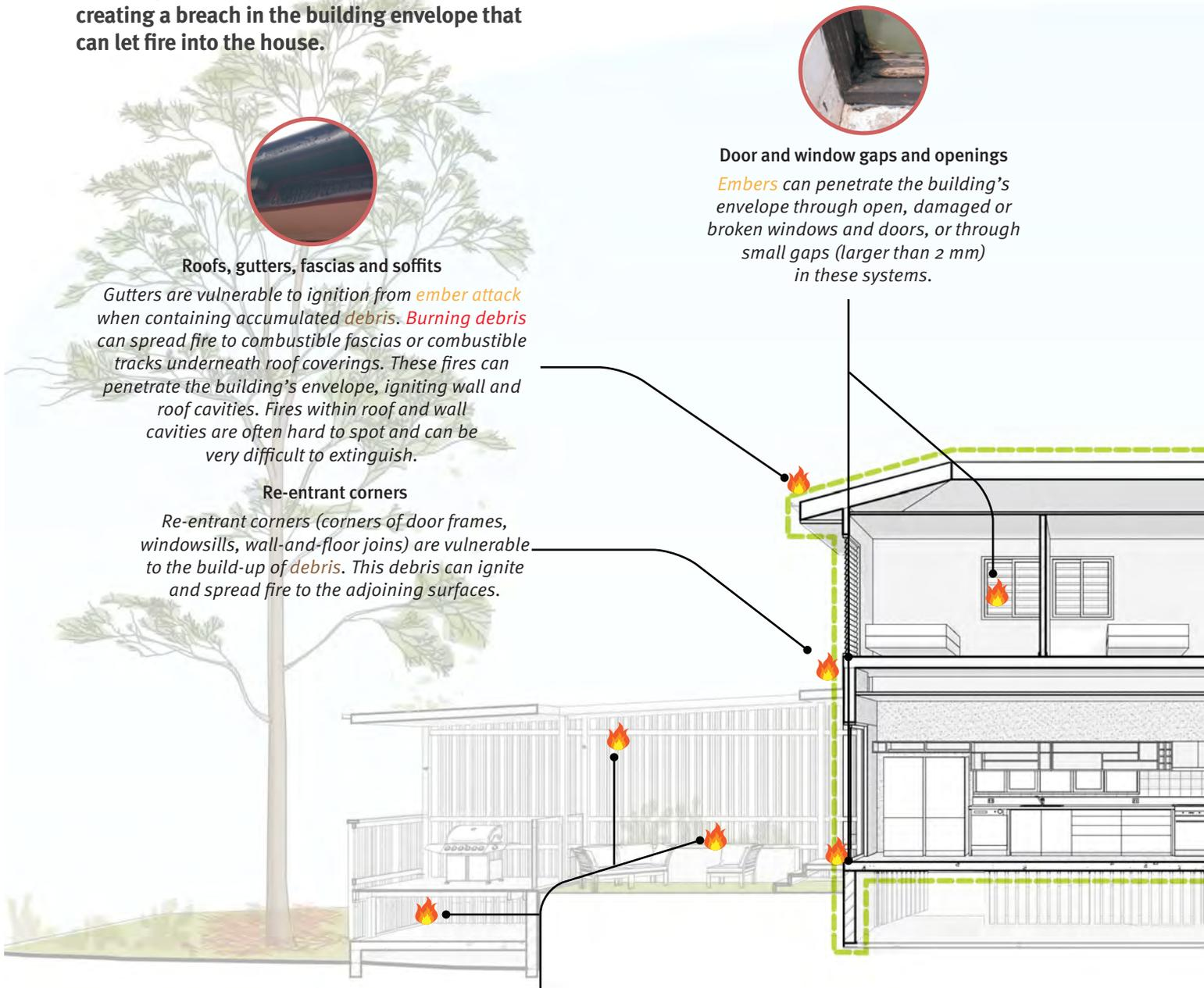
Artificial objects surrounding the house (e.g. decks, fences, sheds, outdoor furniture) are a ready fuel source for consequential fires. These consequential fires produce **radiant heat** and **flame** that can damage vulnerable elements of the house envelope, such as window frames and screens, combustible cladding, air-conditioning units, door frames, post and poles. **Radiant heat**, **flame** and **embers** can then breach the building's envelope through gaps in damaged surfaces.
