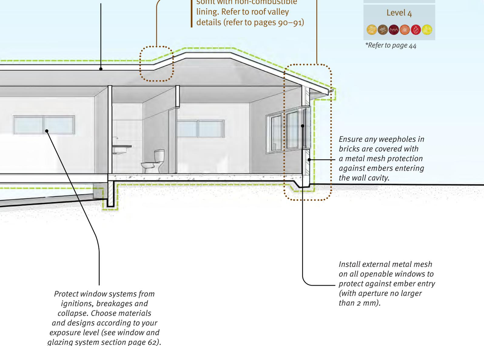
Ensure any weepholes in bricks are covered with a metal mesh protection against embers entering the wall cavity.
