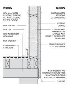
TYPOLOGY: RETROFIT LIGHTWEIGHT WALL TYPE EXTERNAL | EXISTING STUD WALL **FXISTING NON WATER RESISTANT** FLOOR TYPE: FLOOR FINISH ON TIMBER STRUCTURE R-VALUE: RL-203 CODE:
