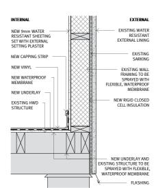
TYPOLOGY: RETROFIT LIGHTWEIGHT EXTERNAL | EXISTING STUD WALL EXISTING NON WATER RESISTANT FLOOR TYPE FLOOR FINISH ON TIMBER STRUCTURE R-VALUE:
