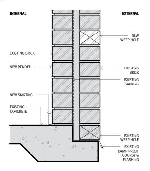
EXTERNAL INTERNAL WEEP HOLE EXISTING BRICK NEW RENDER NEW SKIRTING EXISTING NEW TILE EXISTING NEW WATERPROOF MEMBRANE UNDERLAY EXISTING CONCRETE EXISTING WEEP HOLE EXISTING DAMP PROOF COURSE &
