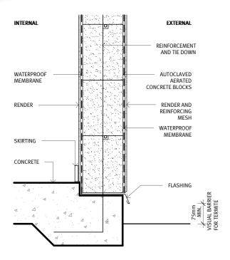
INTERNAL EXTERNAL REINFORCEMENT AND TIE DOWN WATERPROOF MEMBRANE AUTOCLAVED CONCRETE BLOCKS RENDER RENDER AND SKIRTING WATERPROOF MEMBRANE UNDERLAY TILE
