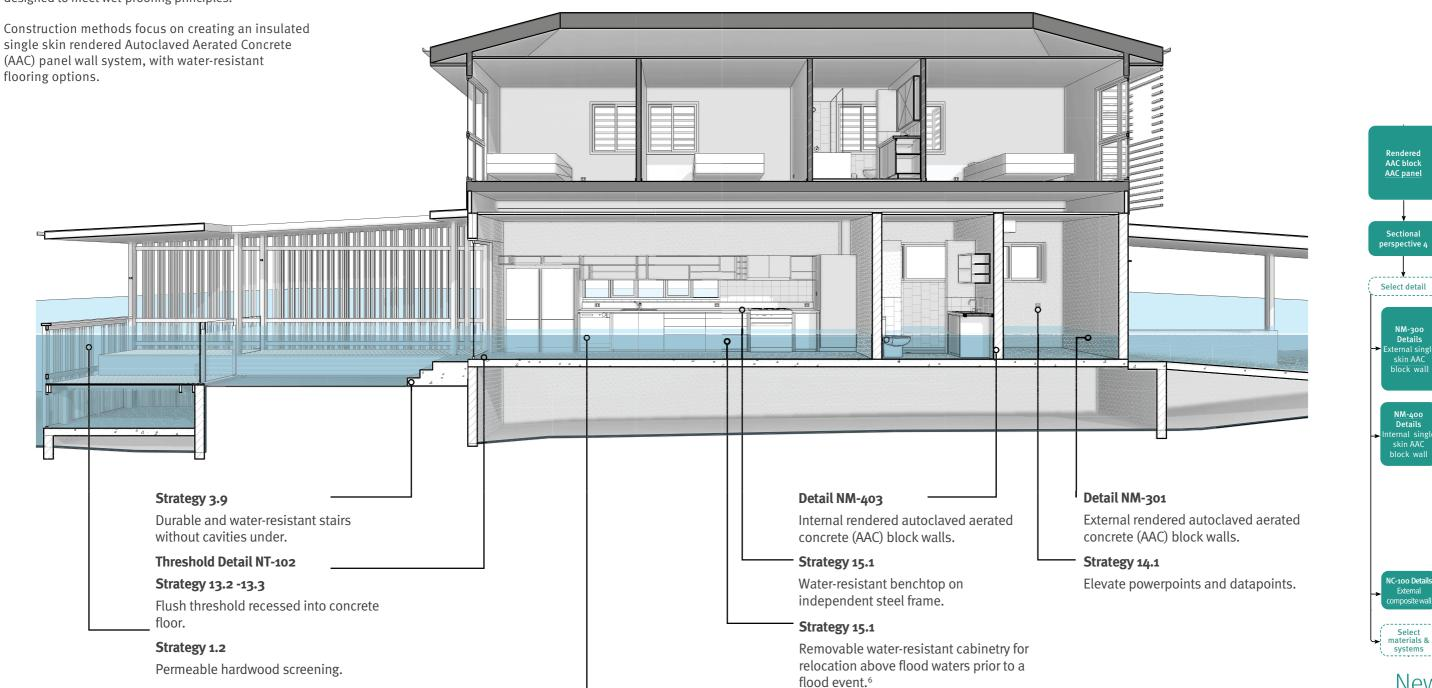
Masonry | Rendered AAC Block
