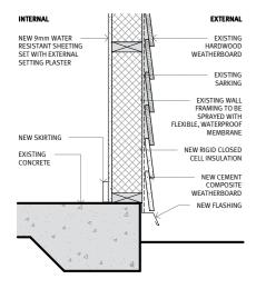
RETROFIT LIGHTWEIGHT TYPOLOGY: EXTERNAL | EXISTING STUD WALL WALL TYPE: FLOOR TYPE: EXISTING CONCRETE SLAB R-VALUE:
