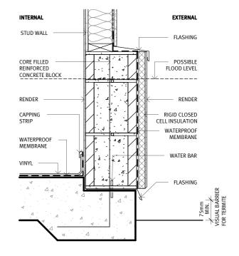
TYPOLOGY: COMPOSITE - LIGHTWEIGHT/MASONRY WALL TYPE: EXTERNAL | CONCRETE BLOCK AND STUD
