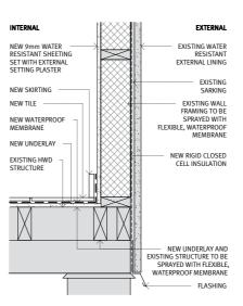
TYPOLOGY: RETROFIT LIGHTWEIGHT EXTERNAL | EXISTING STUD WALL **FXISTING NON WATER RESISTANT** FLOOR TYPE: FLOOR FINISH ON TIMBER STRUCTURE R-VALUE: RL-203 CODE:
