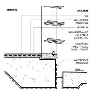
TYPOLOGY: THRESHOLD WALL TYPE: TILE | GROUND FLOOR FINISH: R-VALUE: CODE: NT-104
