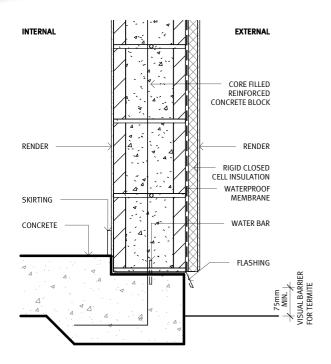
EXTERNAL INTERNAL CORE FILLED REINFORCED CONCRETE BLOCK RENDER RENDER SKIRTING RIGID CLOSED WATERPROOF WATERPROOF MEMBRANE UNDERLAY WATER BAR
