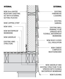
RETROFIT LIGHTWEIGHT TYPOLOGY: EXTERNAL | EXISTING STUD WALL WALL TYPE: FLOOR TYPE: EXISTING NON WATER RESISTANT FLOOR FINISH ON TIMBER STRUCTURE R-VALUE: CODE: RL-104
