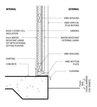
INTERNAL EXTERNAL HWD NOGGING HWD VERTICAL STUD BEYOND RIGID CLOSED CELL SARKING 9mm WATER WATER RESISTANT RESISTANT LINING SET WITH EXTERNAL SETTING PLASTER SKIRTING HWD NOGGING WATERPROOF MEMBRANE HWD BOTTOM UNDERLAY TILE FLASHING \_ \_ \_ \_ \_ \_
