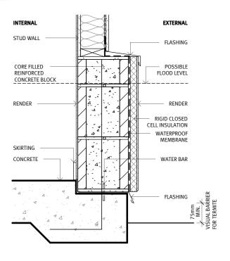
EXTERNAL INTERNAL STUD WALL FLASHING CORE FILLED REINFORCED FLOOD LEVEL CONCRETE BLOCK RENDER RENDER SKIRTING CELL INSULATION WATERPROOF WATERPROOF LINDERI AY WATER BAR TILE
