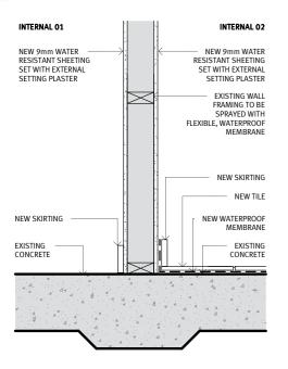
INTERNAL 01 INTERNAL 02 NEW 9mm WATER -RESISTANT SHEETING SET WITH EXTERNAL NEW 9mm WATER SETTING PLASTER SETTING PLASTER FXISTING WALL NFW VINYI FLEXIBLE, WATERPROOF NEW WATERPROOF NEW SKIRTING NFW TILF NEW UNDERLAY NEW WATERPROOF NEW UNDERLAY AND EXISTING STRUCTURE TO BE SPRAYED WITH FLEXIBLE, NEW UNDERLAY WATERPROOF MEMBRANE
