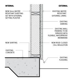
TYPOLOGY: RETROFIT LIGHTWEIGHT EXTERNAL | EXISTING STUD WALL FLOOR TYPE: EXISTING CONCRETE SLAB R-VALUE: RL-201
