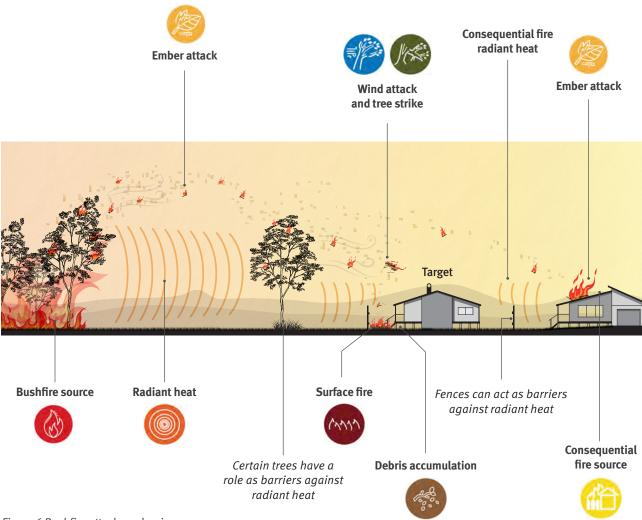
Figure 6 Bushfire attack mechanisms
