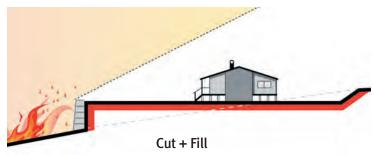
Figure 11 Terracing of sloping ground can block and deflect embers and radiant heat away from buildings (from Caird and Ramsay, 2003)
