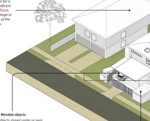
Movable objects stored under or near the house (e.g. cars, boats, wood heaps, wheelie bins) are vulnerable to ignition and can form a consequential fire that may ignite, damage or destroy vulnerable elements of the house.
