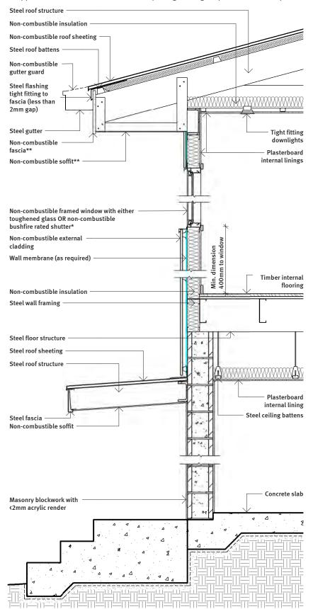
\* For more information refer to AS3959:2018 \*\* Fibre cement sheet of a minimum of 4.5mm or greater to prevent FC distortion
