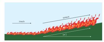
Figure 5 Influence of slope on fire propagation
