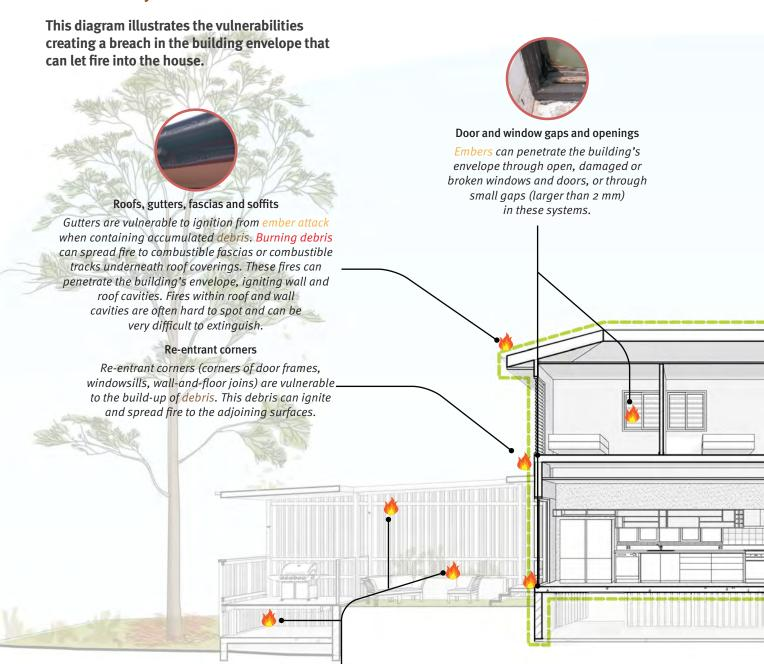
Artificial objects surrounding the house (e.g. decks, fences, sheds, outdoor furniture) are a ready fuel source for consequential fires. These consequential fires produce radiant heat and flame that can damage vulnerable elements of the house envelope, such as window frames and screens, combustible cladding, air-conditioning units, door frames, post and poles. Radiant heat, flame and embers can then breach the building's envelope through gaps in damaged surfaces.
