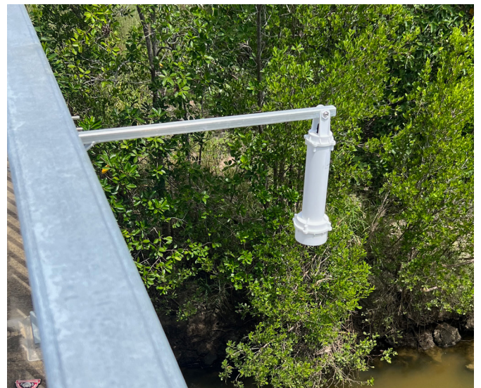
LiDAR water level sensor (Credit: Lixia)
