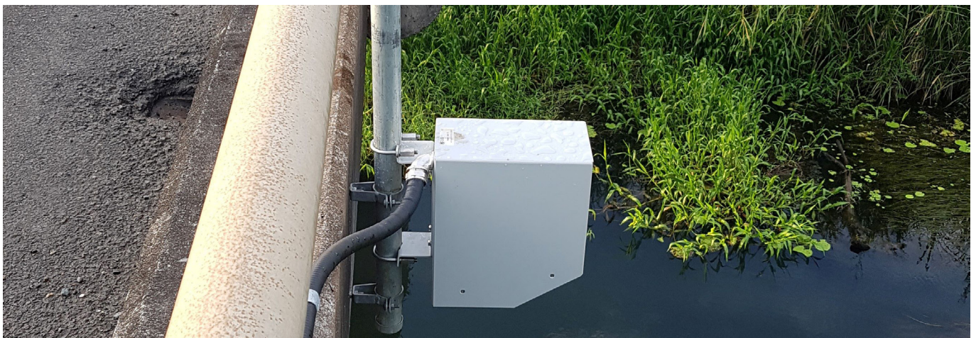
Radar water level sensor (Credit: Sunwater)
