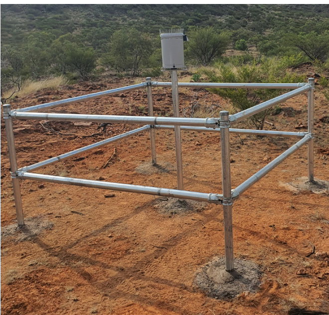
Rainfall gauge with pulse satellite data logger (Credit: Ontoto)
