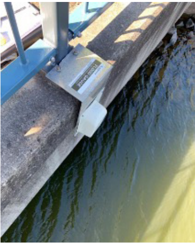
Radar water level sensor (Credit: Sunshine Coast Council and HiLo Level Monitoring)
